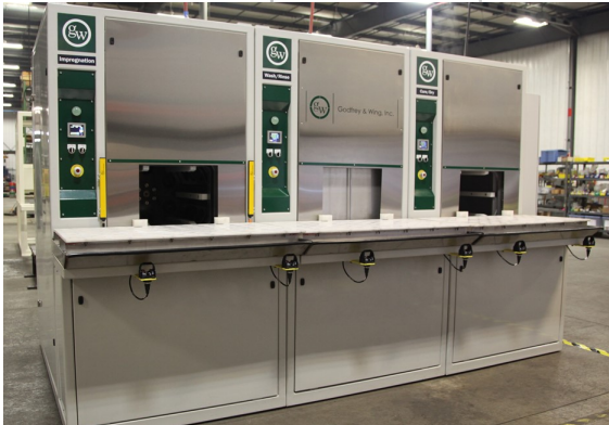
The HVLV's single piece part flow allows for better casting recovery and zero leak rate.
